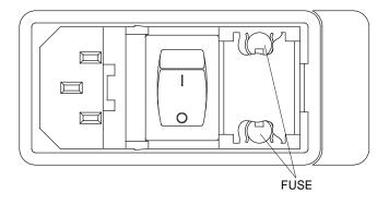
Figure 5-1: AC Fuse Replacement
